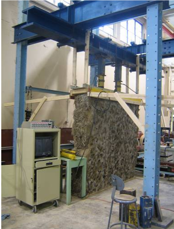
Hemp bale test wall prior to testing.
